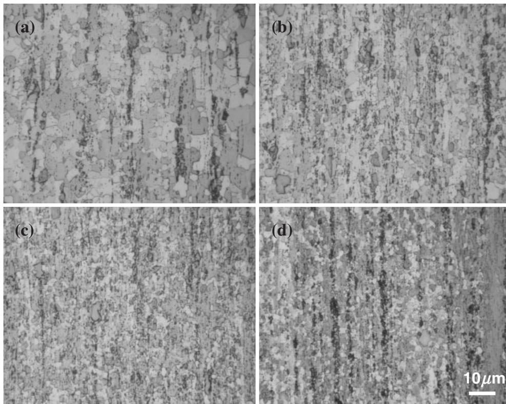
Fig. 3 Optical micrographs of the as-extruded Mg-5Al-3Ca-xY alloys;  $x = 0$  (a), 1 (b), 2 (c) and 3 mass% (d).
