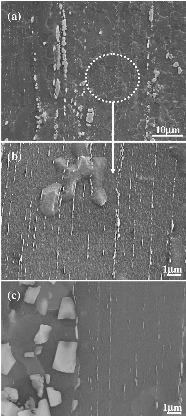
Fig. 6 SEM images in high magnification of the as-extruded alloy: (a) lower magnification, (b) higher magnification and (c) the backscattered image (BEI).
