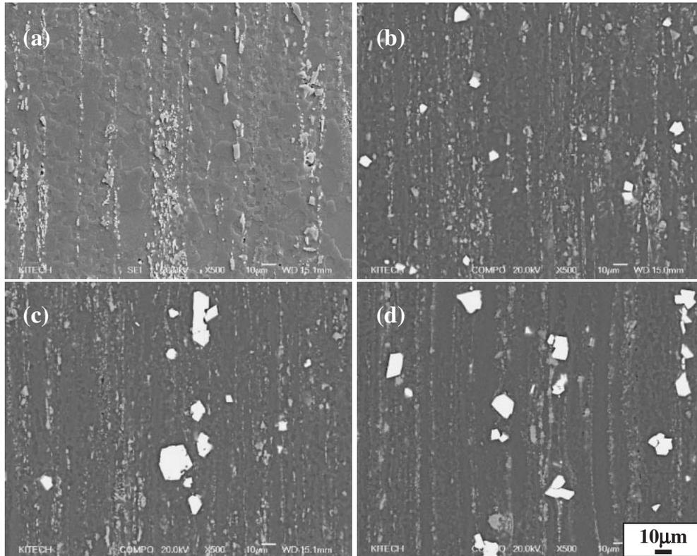
Fig. 4 SEM images of the as-extruded Mg-5Al-3Ca-xY alloys:  $x = 0$  (a), 1 (b), 2 (c) and 3 mass% (d).
