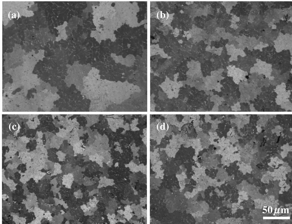
Fig. 2 Macrostructure of as-cast Mg-5Al-3Ca-xY alloys;  $x = 0$  (a), 1 (b), 2 (c) and 3 mass% (d).
