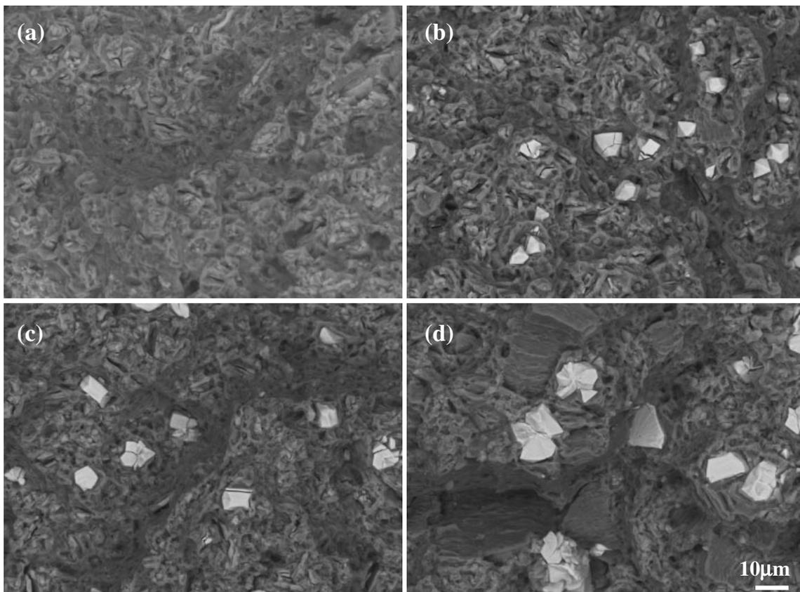
Fig. 9 The backscattered SEM fracture images of the as-extruded Mg-5Al-3Ca- $x$ Y alloys obtained from the tensile test at room temperature:  $x = 0$  (a), 1 (b), 2 (c) and 3 mass% (d).
