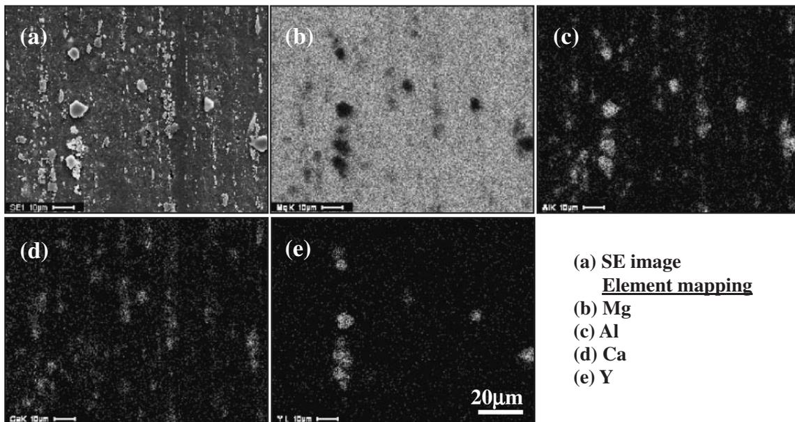
Fig. 5 SEM-EDS element mapping images of the as-extruded Mg-5Al-3Ca-2Y alloy.
