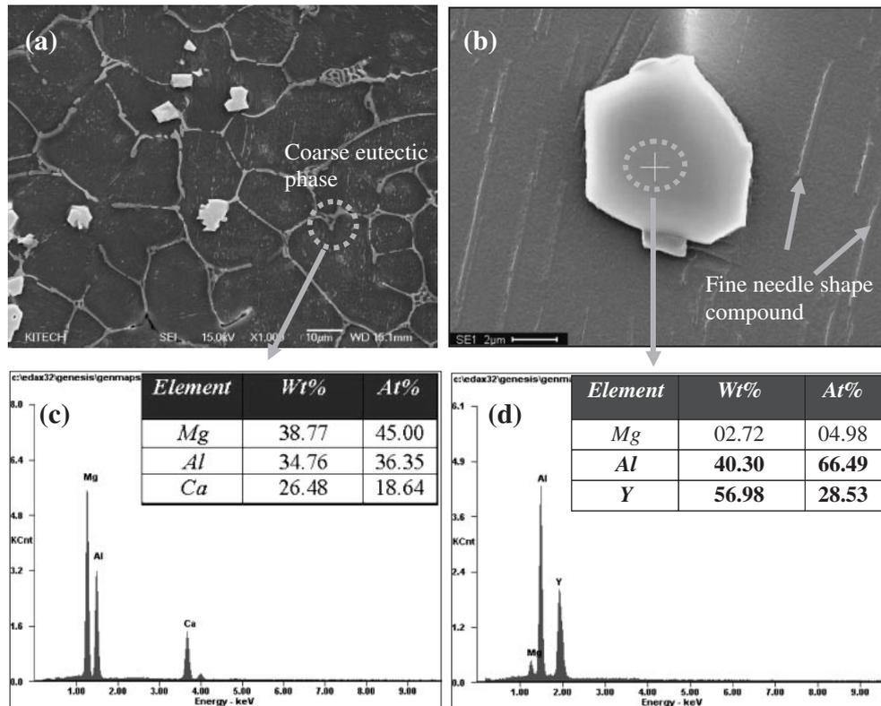
Fig. 1 SEM-EDS analysis of as-cast Mg-5Al-3Ca-3Y alloys; (a), (b) SEM image, (c) EDS result of eutectic phase and (d) EDS result of Y containing intermetallic compounds.
