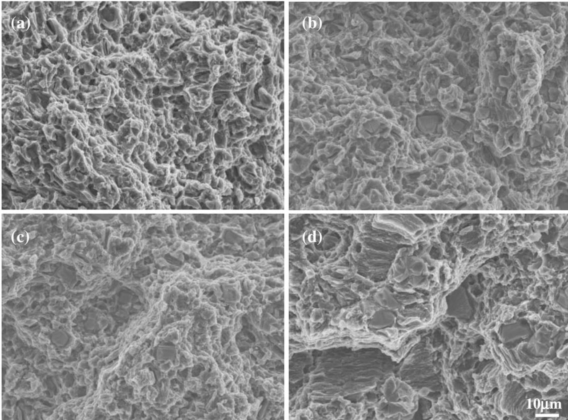
Fig. 8 SEM fracture images of the as-extruded Mg-5Al-3Ca- $x$ Y alloys obtained from the tensile test at room temperature:  $x = 0$  (a), 1 (b), 2 (c) and 3 mass% (d).
