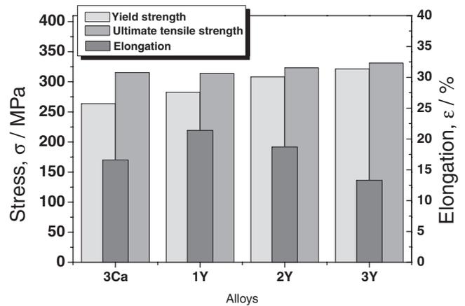
Fig. 7 Tensile properties of the as-extruded Mg-5Al-3Ca-xY alloys at room temperature.
