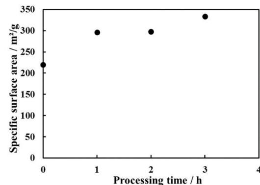
Fig. 6. Result of specific surface area of RHC and each ET-RHC
