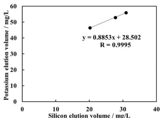
Fig. 4. Relationship between potassium elution volume and silicon elution volume
